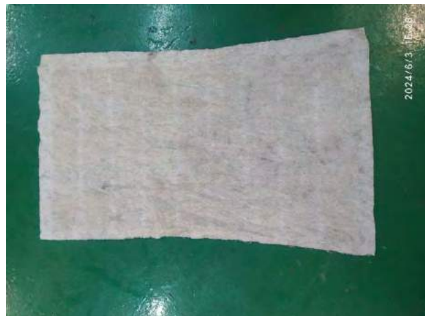
Air filter – Washed and reused
